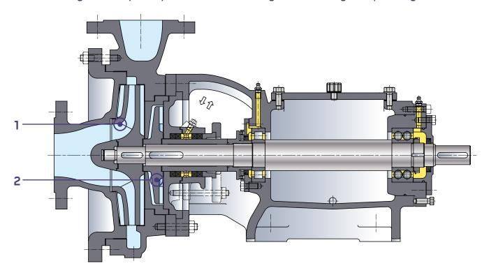
RCE DWH: Heated design with hydrodynamic shaft sealing and ring valve
