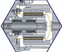
Magnetic coupling Sealed by a spacer can in a range of materials
