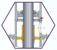
Labyrinth seal Contact-free seal for nonpressurised container systems
